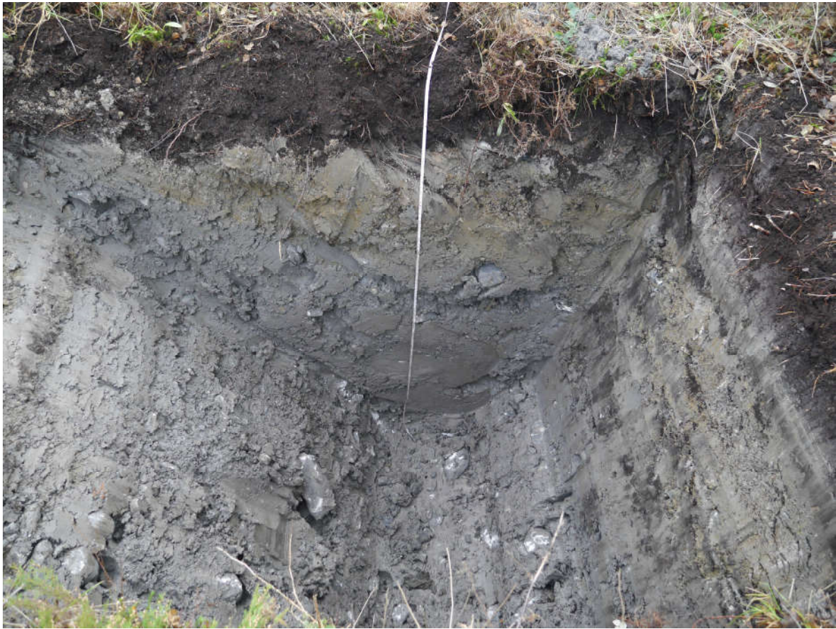
Figure 2-2: Photo through Trial pit (GDG TP101) near T22 showing peat underlain by cohesive glacial till (Photo Dated November 2016)
